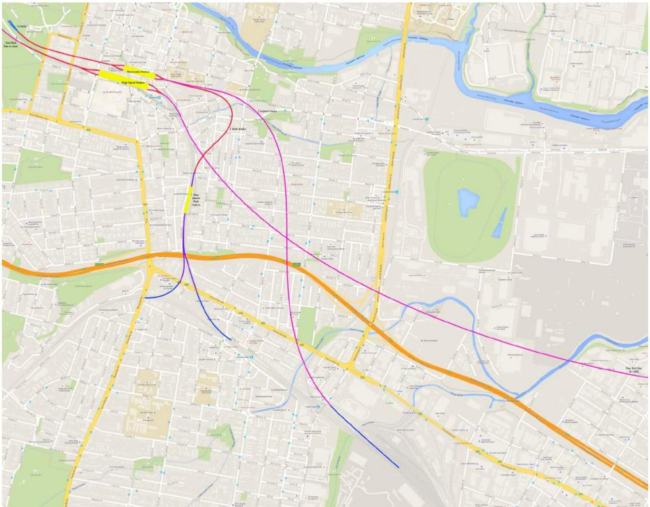
**Stage 3** sees the introduction of long distance High Speed Rail service. Note that the High Speed Rail line involves twin tunnels. Because of their relative depth they will pass under the tunnels created in stage 1A in the general vicinity of Little Street.
